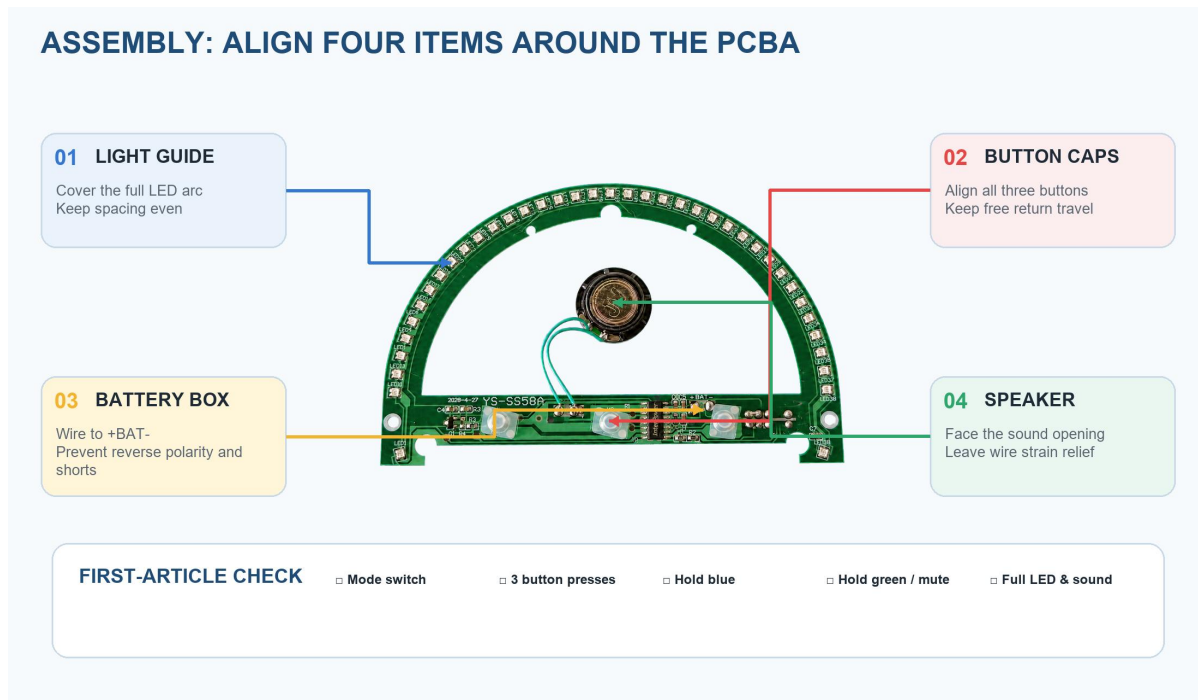
Figure 5. Assembly relationships for the light guide, button caps, battery box and speaker
